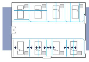
Grosvenor Contracts IV400 lends itself to many configurations within a hospital bed cubicle. The most common configurations of fixed track are shown here, but the specifier should take account of medical factors such as levels of usage, and the possible need of secondary IV provision at the foot of the hed
