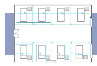
There are several alternatives for IV200 track positions. The most commonly used layout is a track parallel to the back wall and 1m out from it. A continous track is then possible over the line of beds, assuming an unobstructed ceiling. A second track may be positioned across the foot of the beds if required. Another alternative is a track running parallel to the bed. This gives IV provision at both the head and the foot of the bed, and also allows stacking of carriers against a wall.
