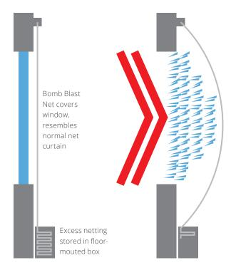
In the instance of an exterior explosion the netting stop dangerous shards of glass entering the room and causing injury
